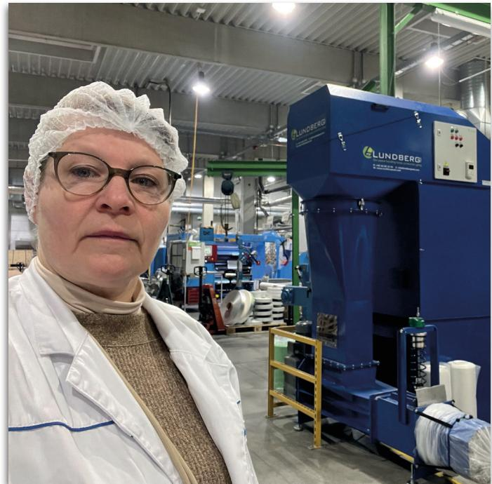
Ms Treder explains: "Before we installed the waste handling units, our waste trims were blown endlessly into large bags, which were difficult and dangerous to transport by forklift. Handling them was also time-consuming and inconvenient due to the low bulk density and frequent transport. The automated waste handling units eliminated these challenges."
